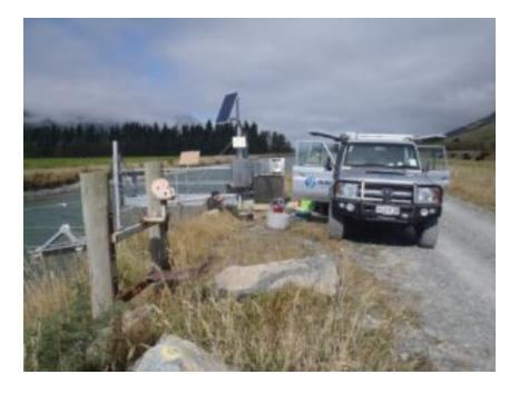
NIWA staff installing an automatic sediment recorder below the gates of the Oakden canal 29 March 2022
